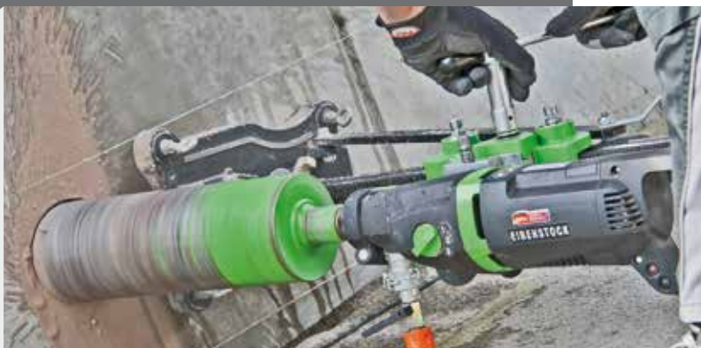
BST 182 V/S: mounted carriage on 4 special balls
