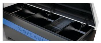
The filtration tank contains four sections with filters to remove oil and fuel deposits.
